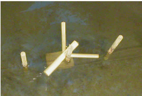
Photograph 1 – A 2B type log trapped on a single pole.
