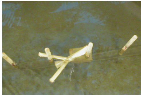
Photograph 2 – A 2B-3D type log trapped between two poles.
